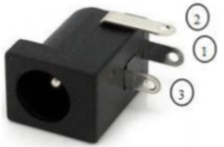
Figure 2: Three-terminal DC barrel jack. In this experiment, only terminal 1 and terminal 3 are used.
